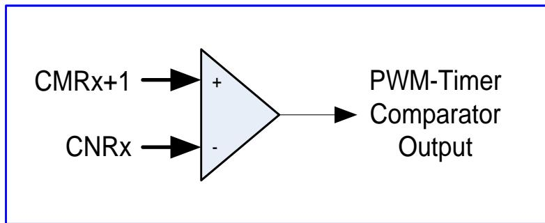
$\text{CMRx+1} \geq \text{CNRx}$ : PWM output high.
