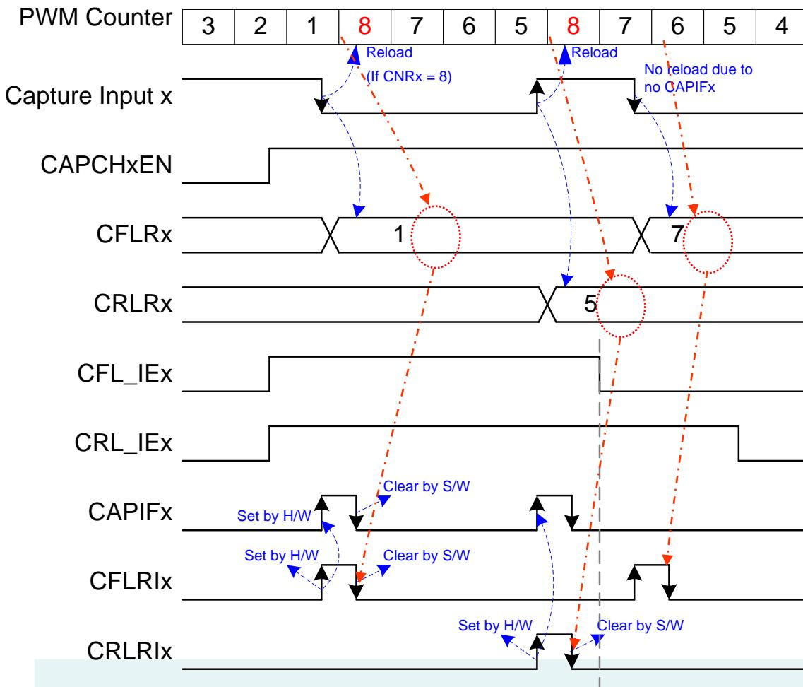
The PWM counter will be reloaded with CNRx when a capture interrupt flag (CAPIFx) is set
